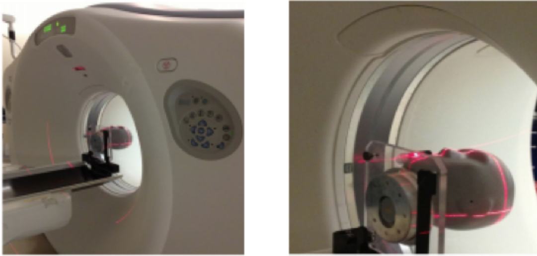
Figure 2.1. Commercial Pediatric Head Phantom in the CT Scanner at the Department of Radiation Medicine, Loma Linda University Medical Center
